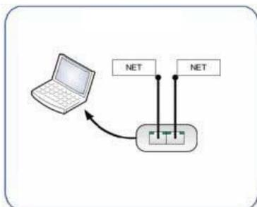
**EtherShark™ Tap** sees and monitors all seven protocol layers, and captures and aggregates **full-duplex** traffic at wire-speed (200Mb).
