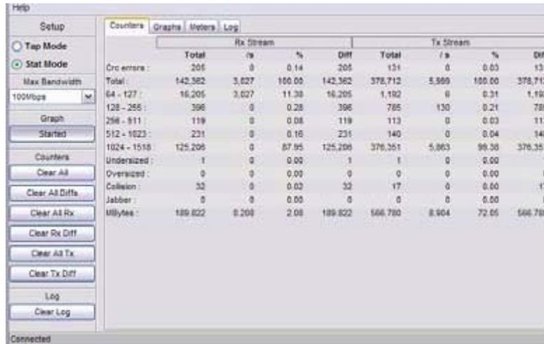
**EtherShark™ Tap** counts the following events: CRC error, size bracket of frames, undersized and oversized frames, collisions and jabbers. Furthermore the lower row gives the total of bytes seen.
