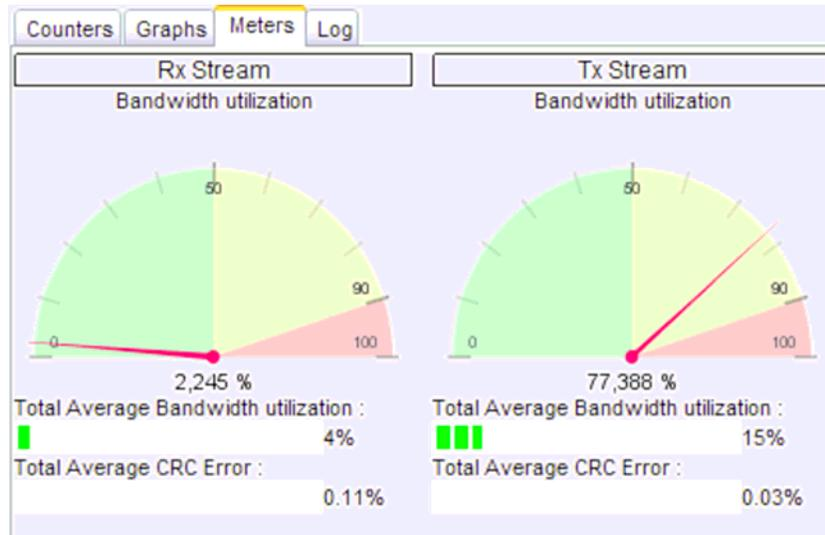
This view use meters and gauges to display the average bandwidth utilization, and CRC error occurrences. The values are percentage of the total of seen packets on the monitored TX and RX lines.
