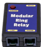
Relay Closure on Ring Voltage
